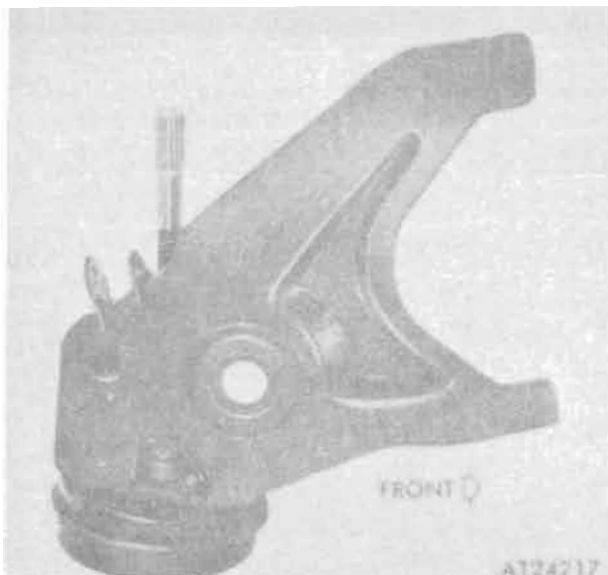
Figure 11-2. Rear Suspension Arm Assembly—Bottom View (M151A2, M825, and M718A1 Vehicles).
