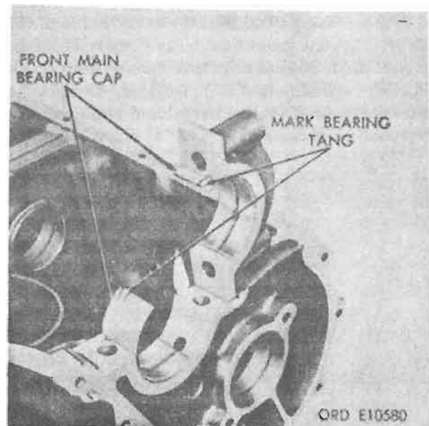
Figure 4-224. Main bearing installation.
