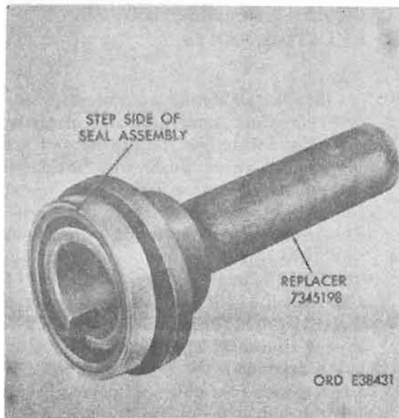
Figure 4-195. Oil seal assembly installation on replacer tool, 7345198.
