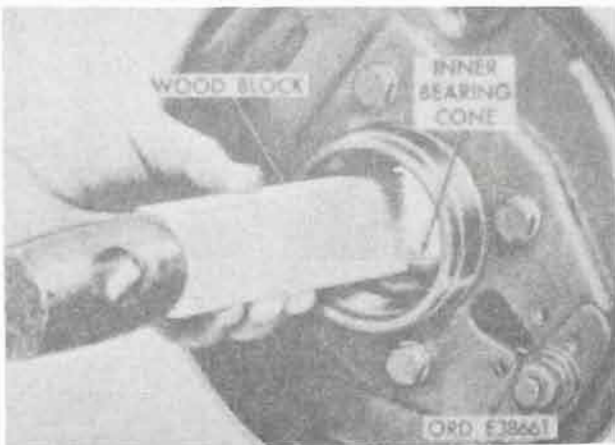
Figure 10-48. Driving inner bearing cone to loosen bearing seal.
