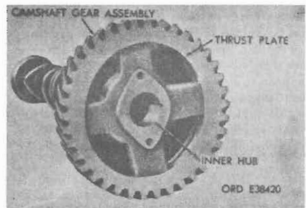
Figure 4-177. Camshaft gear installation.
