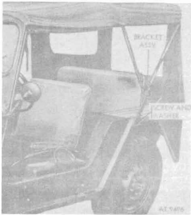
Figure 18-75. Removal of soft top bows and brackets.
