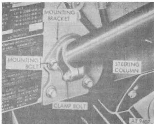
Figure 16-3. Steering column mounting bracket and attaching hardware (M151, M151A1, M151A1C, and M718 vehicles).
