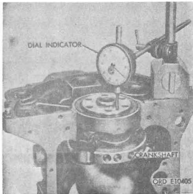
Figure 4-111. Measuring crankshaft end play.
